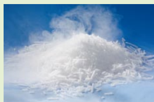
Pellets diameter 3 mm (suitable for dry ice blasting)
